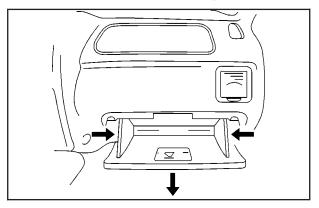
Lower the glove box door, then push in the sides of the glove box to completely lower the door to allow access to the slot where the air filters will be installed.
